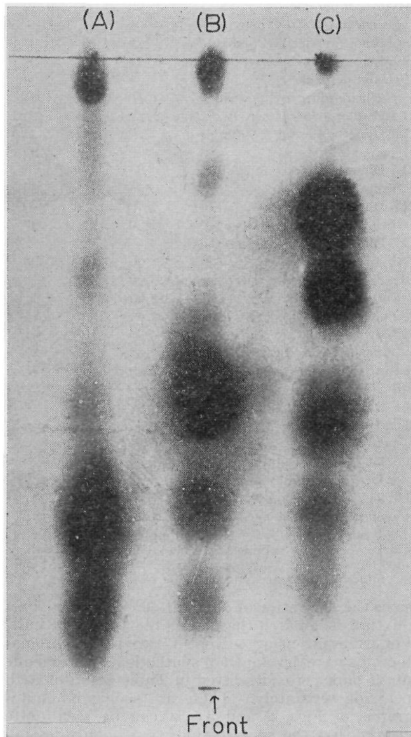
Fig. 1.—Paper chromatogram of ketone peroxides, 80 \gamma (crude): (A) from heptanone-2, (B) from diethyl ketone, (C) from methyl ethyl ketone.
